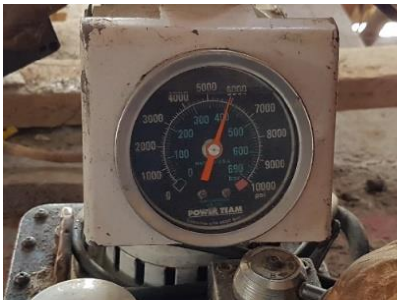
Figure 91: Pressure gauge marking 400 Bar.
